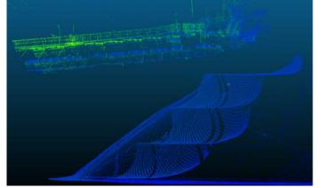
3D scan data from a single scanning system mounted on top of the machine apex (side view of machine boom and bench profile, ground to top layer)
