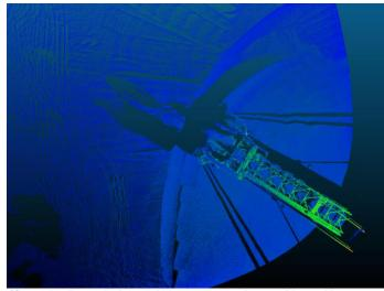
*3D scan data from a single scanning system mounted on top of the machine apex (top view of machine boom, bench profile and even dozer imprints on top of pile)*
